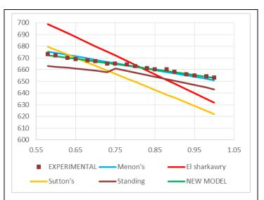
Figure 1: Comparison of Pseudo critical temperatures versus Specific gravity
